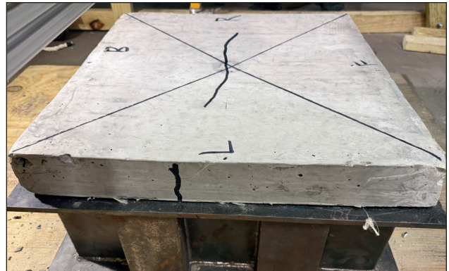
1st impact: 54 lb. weight. 8' drop on concrete reinforced with SafeTcrete fiber. No rebar. Minor fissures appear on all edges and top.
