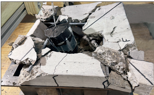
4th impact: 54 lb. weight. 8' drop on concrete reinforced with steel rebar, 12" center. Complete failure by fragmentation. Large pieces ejected from all sides.
