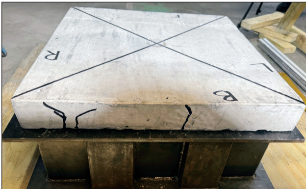
1st impact: 54 lb. weight. 8' drop on concrete reinforced with steel rebar, 12" center. Minor fissures appear on all edges. Slight chipping on back.
