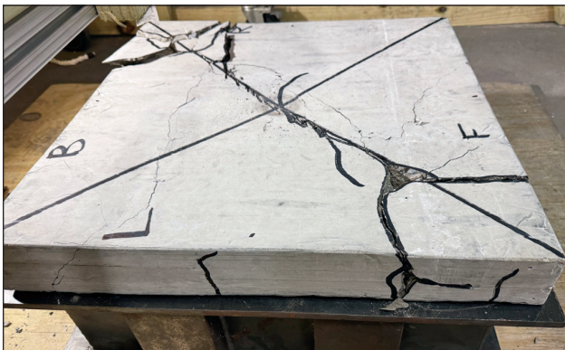
3rd impact: 54 lb. weight. 8' drop on concrete reinforced with steel rebar, 12" center. More fissures. Some have become significant crevices, extending across top to join others. Some fragmentation has occurred leaving two corners detached from the slab.
